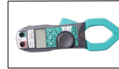
Rajah 4.12: Clamp-on Meter
