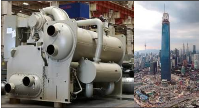
Rajah 2.8: Renesas Semiconductor KL Sdn. Bhd. (July 2017) & TRX Building (7 units of R1233zd chillers)
