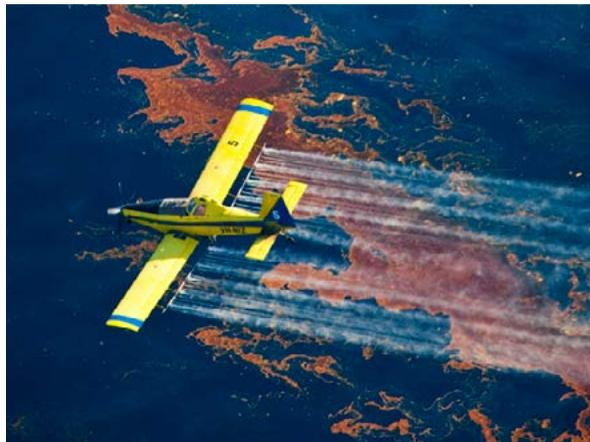
**Figure 3:** Deployment Using Aircrafts (Photo source: Mark Hamilton Photography)
