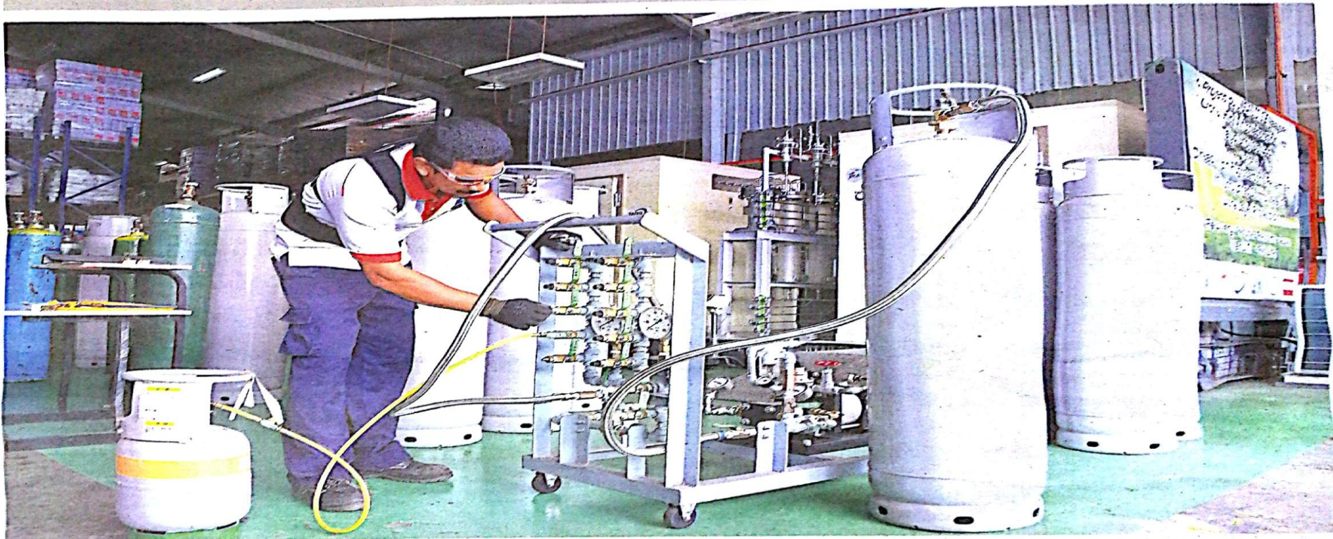
Green initiative: An employee at Westech Chemicals Sdn Bhd's reclamation facility transferring recycled fluorocarbons into smaller cylinders as part of the pilot project, which enables users to sell the collected gases and buy back the recycled and reclaimed gas at two-thirds of the market price. — SYED AZAMUDDEN/The Star
