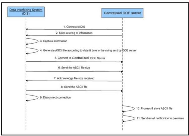
Figure 3.2: General flow diagram
