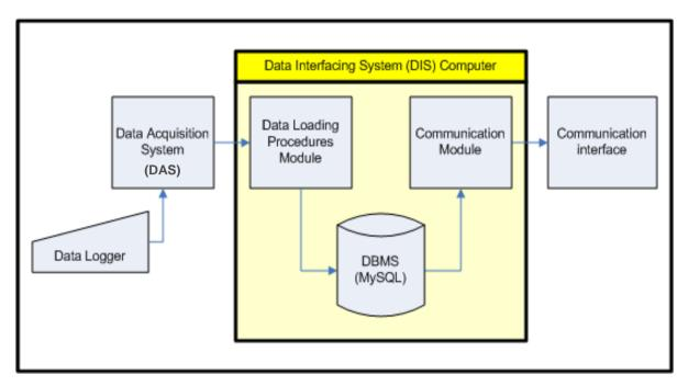
Figure 3.1: CEMS-Data Interfacing System (DIS) Components
