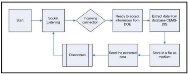
Figure 3.3: Workflow for Communication Procedure via Internet
